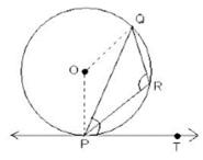
$m \angle OPT = 90^{\circ}$  (:: radius is perpendicular to the tangent)
