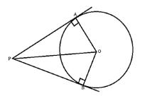
Let P be an external point and PA and PB be tangents to the circle. We need to prove that PA = PBNow consider the triangles  $\triangle OAP$  and  $\triangle OBP$   $m \angle A = m \angle B = 90^{\circ}$  OP = OP [common] OA = OB = radii of the circleThus, by Right Angle- Hypotenuse- Side criterion of congruence we have  $\triangle OAP \cong \triangle OBP$ The corresponding parts of the congruent triangles are congruent, Thus, PA = PB
