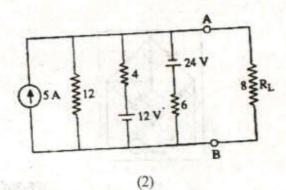
Determine the current flowing through the 5&! resistor in the circuit shown in Fig. by using Norton's theorem.
