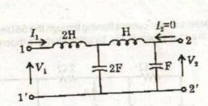
Find the Z-parameters for the network shown in Fig. given below
