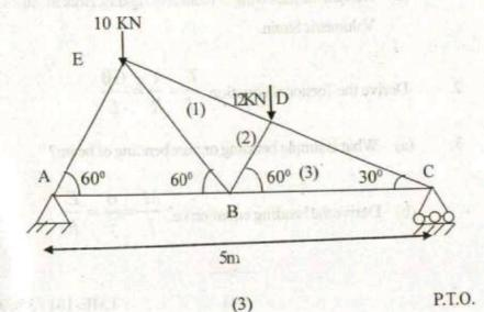
3. Draw shear force and bending moment diagram
