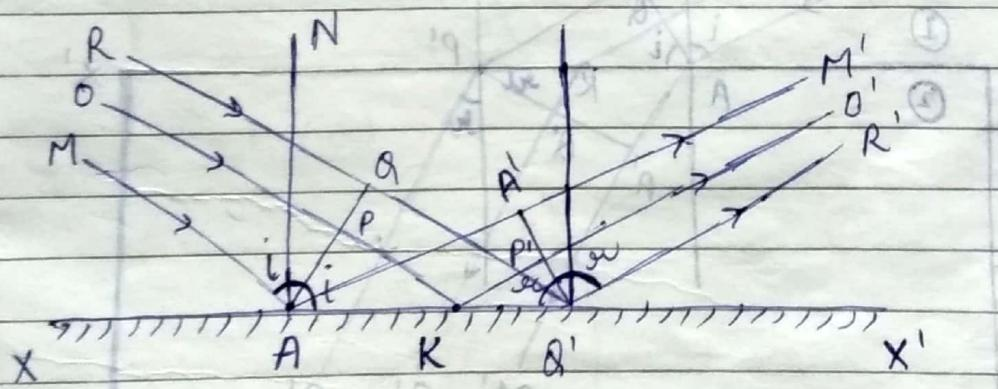
Time taken by a wave to reach from P - P' via K can be given as
