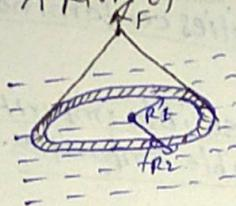
$$F = T \cdot 2\pi R_1 + T \cdot 2\pi R_2 \\ = 2\pi T (R_1 + R_2)$$
