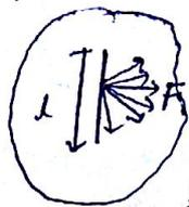
$$T \text{ or } \sigma = \frac{F}{L} \Rightarrow \text{Act } \perp \text{ to line assumed.}$$
