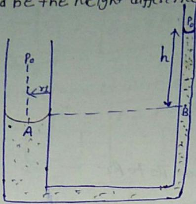
$$h = \frac{2T}{\rho g} \left( \frac{r_1 - r_2}{r_1 r_2} \right)$$
