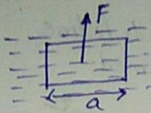
$$F = \text{Force on one surface} \times 4 \\ = (T \times 2a) \times 4 \\ = 8TA$$
