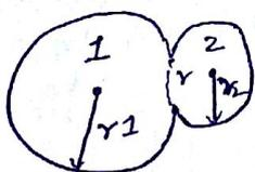
$$r = \frac{r_1 r_2}{r_1 - r_2}$$
