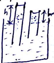
iiii) → If capillary is inclined at angle ' $\theta$ ' with vertical.
