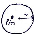
$$P = P_{in} - P_{out} = \begin{cases} \frac{2\sigma}{r} & \text{For one free surface.} \\ \frac{4\sigma}{r} & \text{For two free surface.} \end{cases}$$
