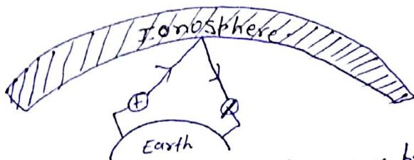
\*\* Critical freq (c) → Max freq. of sky wave propagation up to that the reflection from ionosphere will detect place or just after that signal is reflected.
