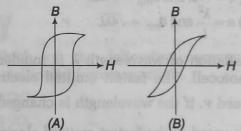
These materials are used to make magnets for electric generators, transformer core and electromagnet core. Then, it is proper to use
