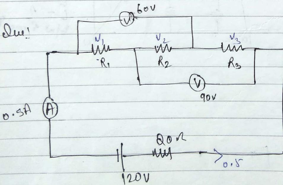
$$V_1 + V_2 = 60$$
