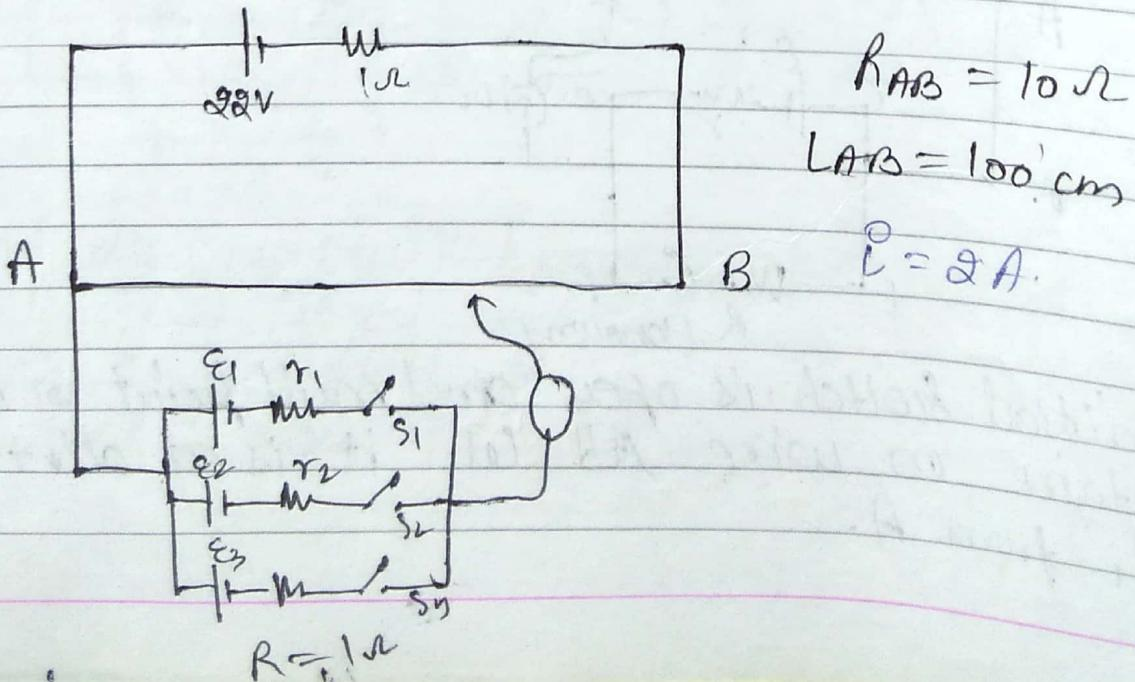
(i) When only  $S_1$  is closed, null point at 80 cm from A when  $S_1$  and  $S_3$  are closed then null point at 40 cm from A find  $E_1$  and  $R_1$ .
