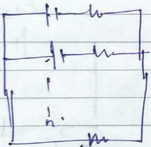
$$E_{eq} = \frac{\frac{E_1}{r_1} + \frac{E_2}{r_2} + \frac{E_3}{r_3} + \dots}{\frac{1}{r_1} + \frac{1}{r_2} + \frac{1}{r_3} + \dots}$$
