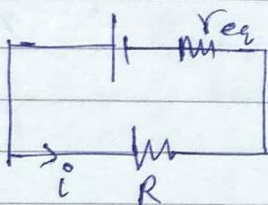
$$\begin{aligned} I &= \frac{E_{\text{eq}}}{R + r_{\text{eq}}} \\ &= \frac{nE}{R + \frac{n r}{m}} \end{aligned}$$
